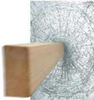
**Proven protection.** Before any window or door product can be certified as impact resistant it must go through a battery of difficult tests. First the unit must go through extensive air and water testing. The second round of tests simulates flying debris by shooting a 2 x 4 at the window from a high-powered air cannon. Finally, the unit goes through intense cycles of positive and negative loads of pressure. If all tests are passed, then the product can become certified.
