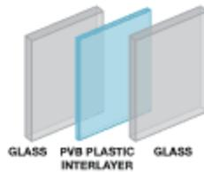
**Fortified glass.** Up to four times stronger than traditional glass, StaySafe's laminated glass features a tough interlayer of .090" gauge KeepSafe® Maximum polyvinyl butyral (PVB) that resists impact from flying debris and traps shards of broken glass. Strong sealants keep the glass from breaking away from the frame.
